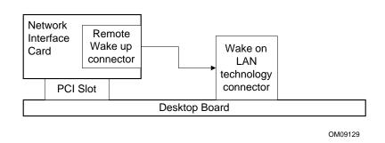
Figure 5. Using the Wake on LAN Technology Connector
